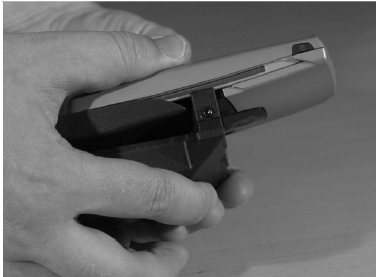
Figure 7: Connecting FLA-21 to Nokia 7650 so that plastic nails attach firmly into tracks.
