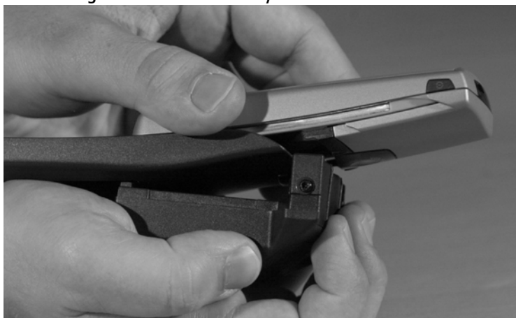
Figure 6: Connect battery connector to FLA-21:
